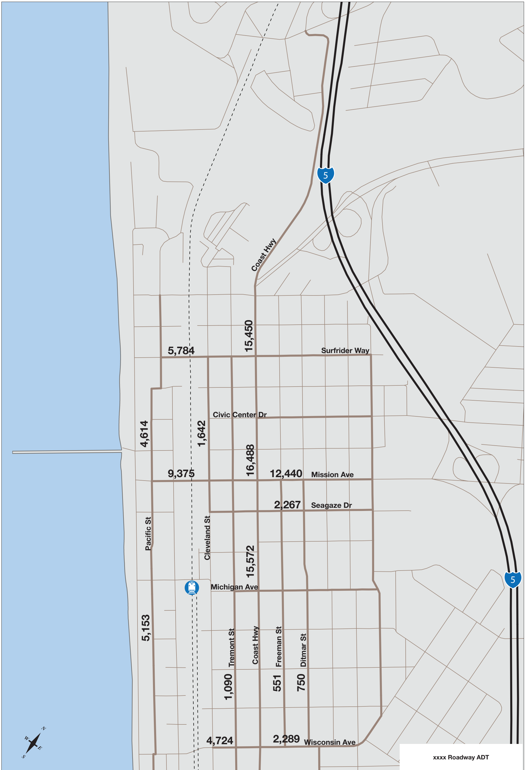
FIGURE 3.2A EXISTING ROADWAY ADT
